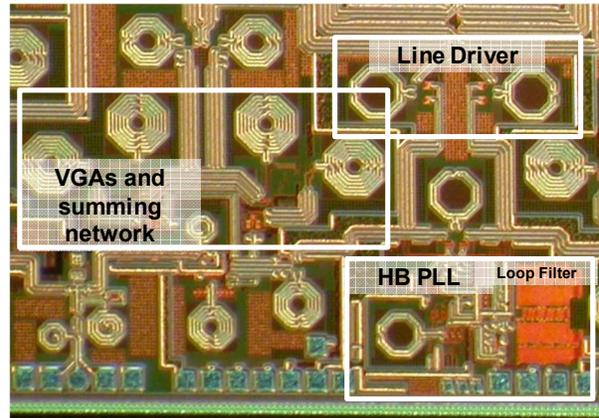
Fig. 7: Die photograph of the high-band synthesizer
