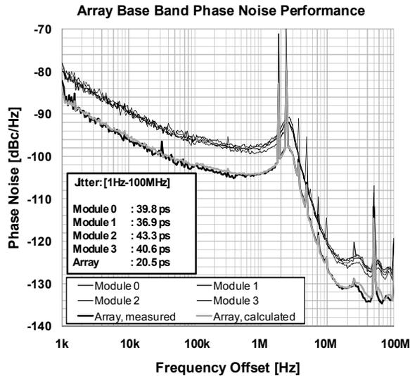
Fig. 6: Measured phase noise at 7.5GHz RF frequency of an *electrical* 4-element array and the individual modules. Spurious tones originate from two of the modules, and are likely related to the custom packaging. Base-band RMS jitter is also shown.
