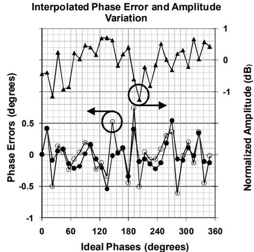
Fig. 5: Phase errors and amplitude variation at  $f_{LO2}=6\text{GHz}$ . Left axis: interpolated phase errors in degrees (dots for integrated- and circles for differential errors). Right axis: normalized amplitude in dB (filled triangles).
