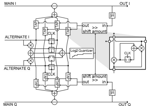
Fig. 6 Enhanced NLMS adaptive equalizer block diagram.
