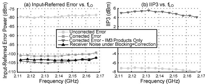
Fig. 8 Measured modified two-tone performance of the receiver, swept over LO frequency. At LNA input TX power is -26dBm, CW power is -34dBm.
