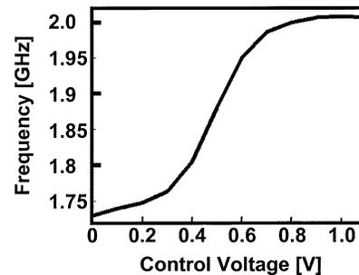
Fig. 15. Quadrature NMOS-only cross-coupled oscillator frequency tuning.
