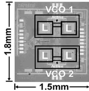
Fig. 14. Quadrature NMOS-only cross-coupled oscillator die photo.
