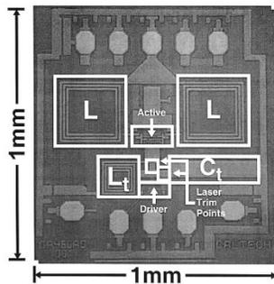
Fig. 11. Differential Colpitts oscillator die micrograph.
