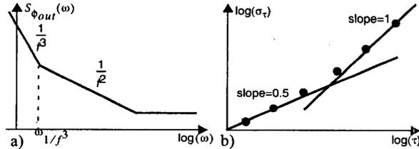
Fig. 4. Typical a) phase noise and b) timing jitter of a free running VCO.
