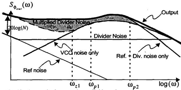
Fig. 12. Phase noise increase due to divider noise.
