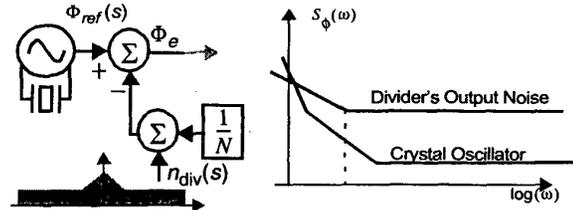
Fig. 11. Equivalent model for frequency divider noise.
