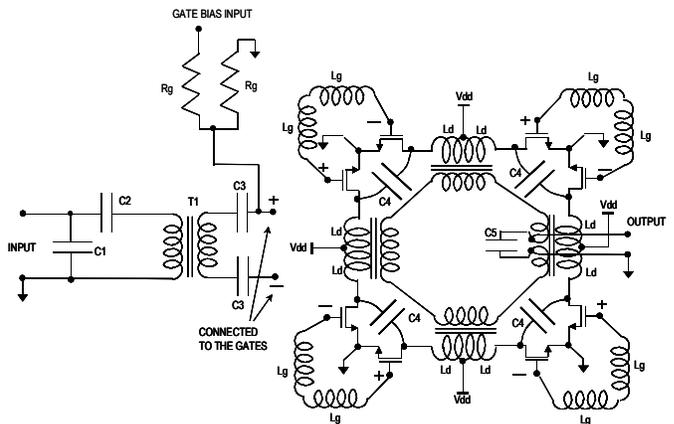
Figure 7- Electrical diagram of circular geometry power amplifier.
