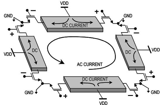
Figure 3- Four Push-pull amplifiers in circular geometry
