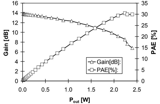
Figure 8- Output Power vs. Gain and PAE with 2V Supply
