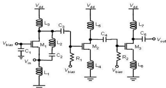
Figure 4. Schematic of LNA
