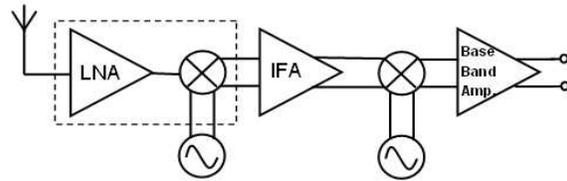
Figure 1. Block diagram of a 24GHz receiver
