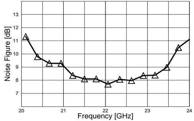
Figure 10. Noise figure (LO frequency = 16.9 GHz)
