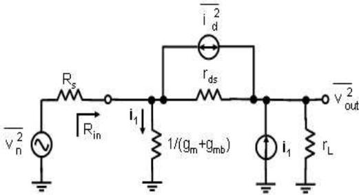
Figure 3. Small-signal model for analyzing the common-gate LNA
