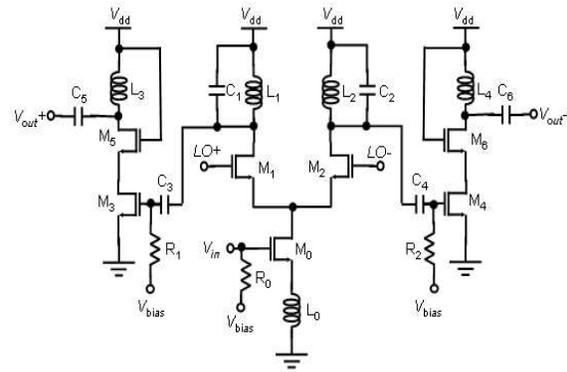
Figure 6. Schematic of Mixer
