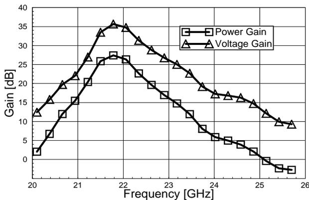
Figure 9. Power gain and voltage gain (LO frequency = 16.9 GHz)
