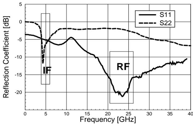
Figure 8. Measured input and output return losses
