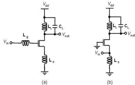
Figure 2. Input Stage (a)common-source with inductive degeneration. (b)common-gate.
