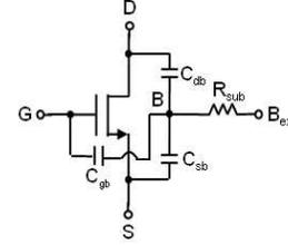
Figure 5. MOSFET substrate network model
