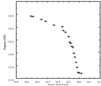
Figure 10. Current-steering delay-balanced tuning in 12 GHz DVCO
