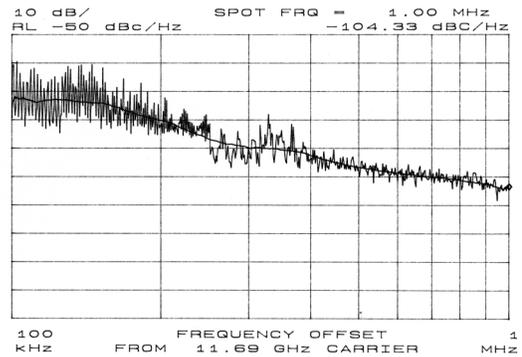
Figure 6. Phase Noise of 12 GHz DVCO
