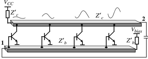
Figure 1. Basic distributed oscillator structure
