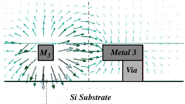
Figure 3. Electric field distribution from HFSS simulation
