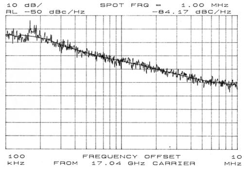
Figure 8. Phase Noise of 17 GHz DVCO
