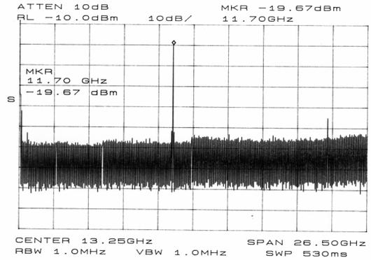
Fig. 5 Power Spectrum of 12 GHz DVCO
