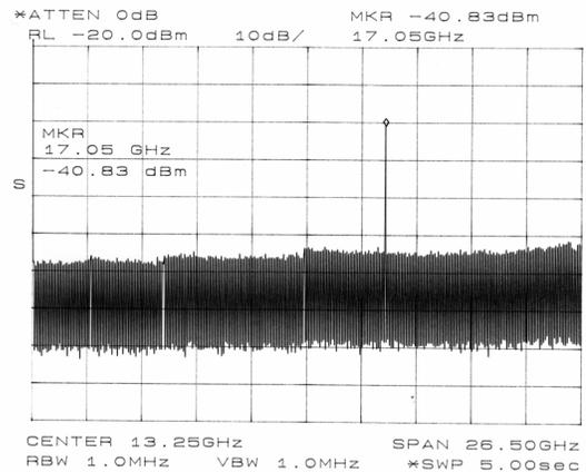
Figure 7. Power Spectrum of 17 GHz DVCO
