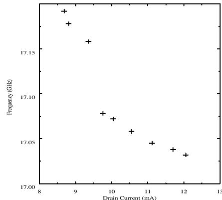
Figure 11 Bias current tuning in 17 GHz DVCO
