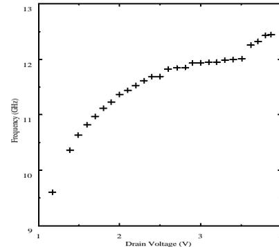
Figure 9. Drain bias tuning in 12 GHz DVCO
