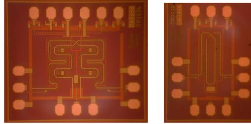
Figure 4. Chip photo: 12 GHz (left), 17 GHz (right)
