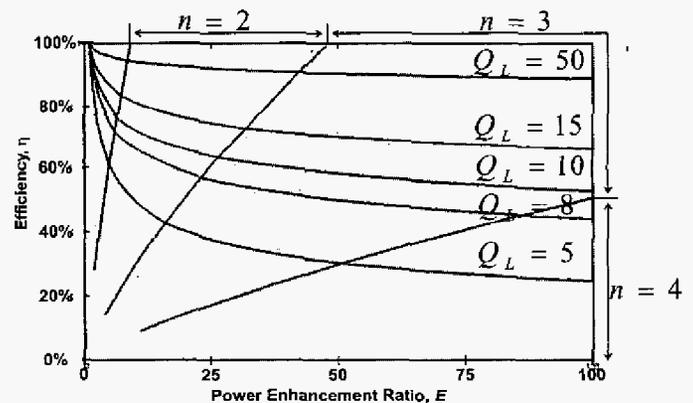
Figure 5. Passive efficiency vs. PER for different inductor  $Q$  in a resonant impedance transformation network with the optimum number of stages.
