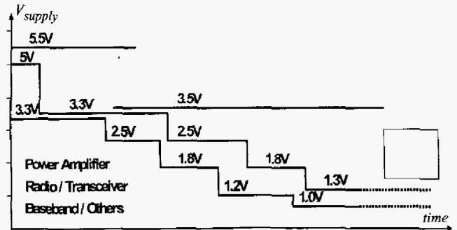
Figure 3. Supply voltage trends in cellular phone building blocks.
