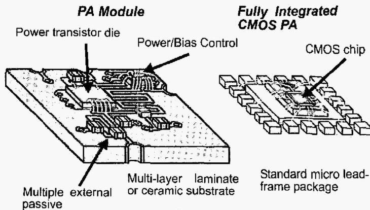
Figure 2: Evolution of PA technology: a) PA modules b) fully integrated CMOS PA
