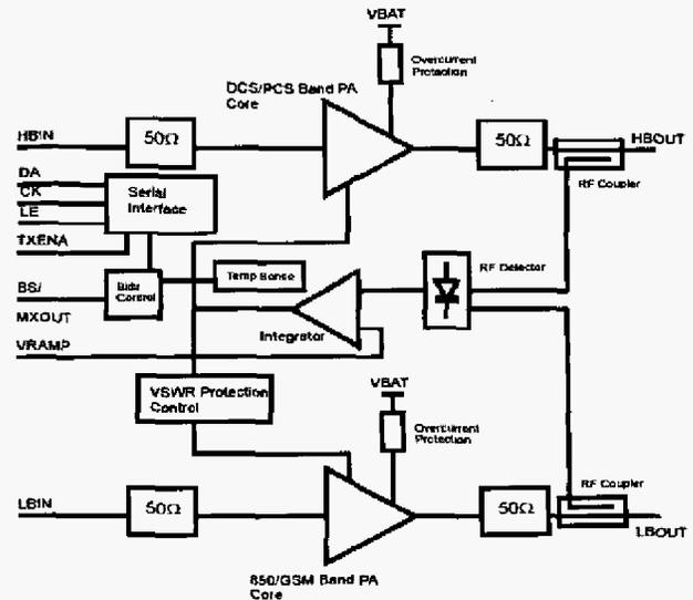
Figure 7. Block diagram of the CMOS fully-integrated power amplifier.
