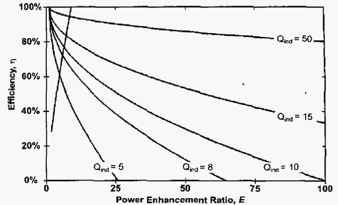
Figure 4. Passive efficiency vs. PER for different inductor  $Q$  in a single-section resonant impedance transformation network.
