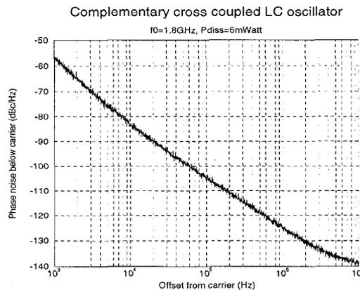
Fig. 6. Phase noise vs. offset frequency for  $V_{dd}=1.5\text{V}$  and  $I_{tail}=4\text{mA}$
