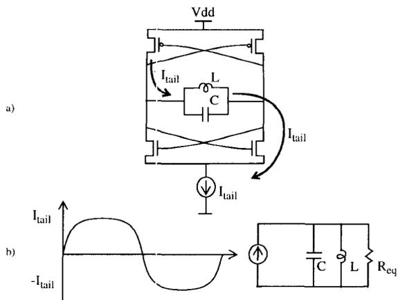
Fig. 2. a) Current flow when the stage is switched to one side b) differential equivalent circuit.
