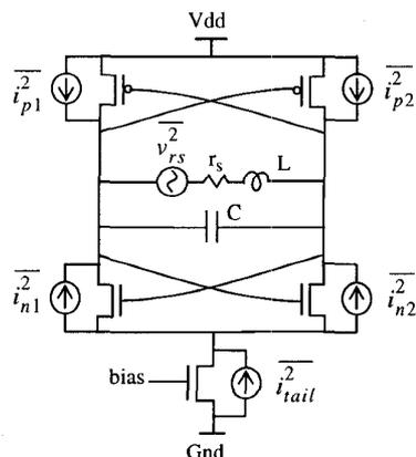
Fig. 3. Complementary LC oscillator with noise sources.
