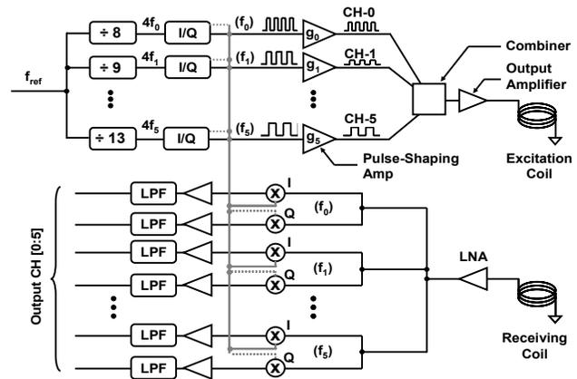
Fig.3: Architecture of the spectral scanning MRI chip.
