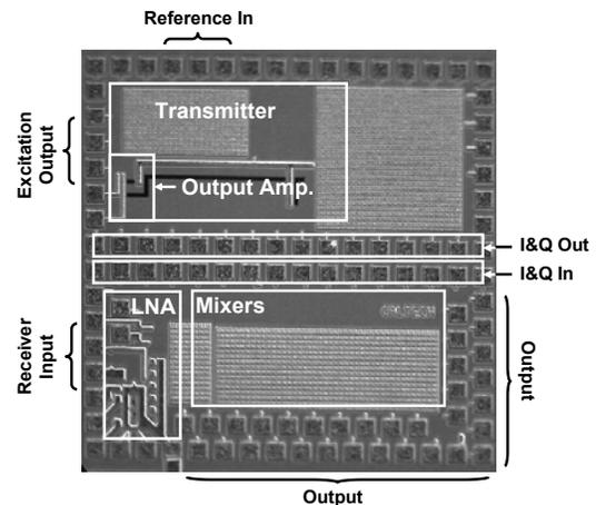
Fig. 4: Chip micrograph
