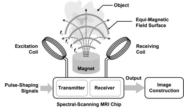
Fig 2: The block diagram of the spectral scanning MRI system, where equi-magnetic field surfaces translate to specific MR resonance frequencies.
