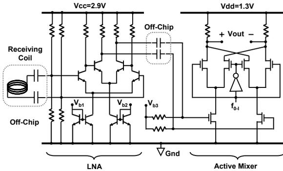
Fig.9: The receiver circuitry for a single channel.
