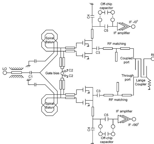
Fig. 1. A simplified schematic of the designed image-rejection subharmonic resistive mixer with integrated IF amplifiers. The IF amplifiers consist of three-stage cascaded resistive feedback inverters.
