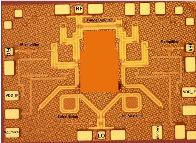
Fig. 2. Micrograph of the realized CMOS subharmonic I/Q mixer.
