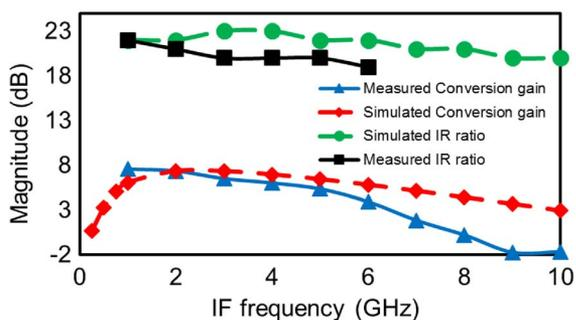
Fig. 6. Measured and simulated conversion gain of I-channel and IR ratio as a function of the IF frequency. The LO was fixed at 85 GHz and RF was swept from 170 to 180 GHz.
