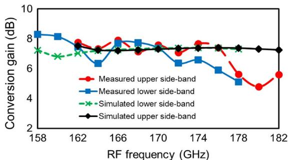
Fig. 5. Measured and simulated upper and lower side-band conversion gain of I-channel at a fixed IF frequency of 2 GHz when the LO was swept from 80 to 90 GHz using a +4 dBm LO power.
