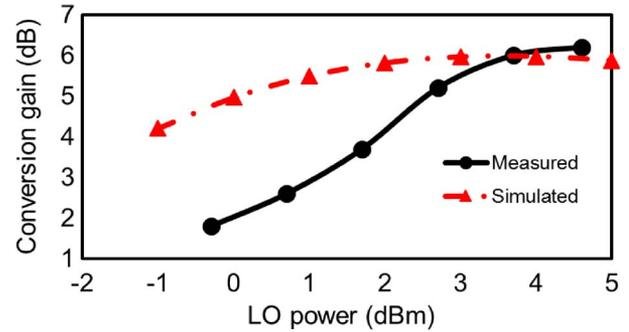
Fig. 3. Measured and simulated conversion gain of Q-channel as a function of LO-power at a fixed LO and RF frequency of 85 GHz, and 172 GHz, respectively.
