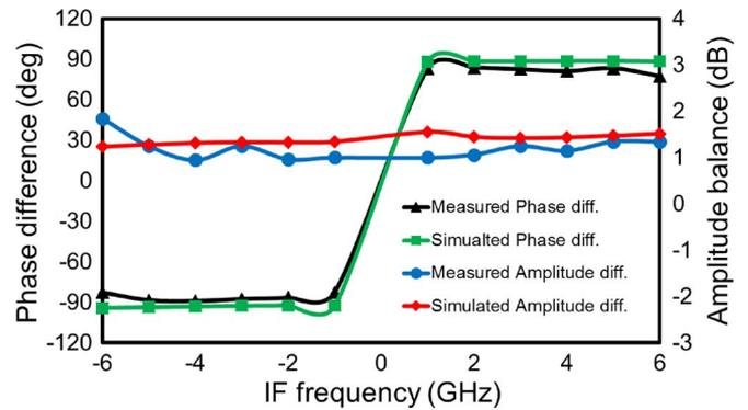
Fig. 4. Measured and simulated quadrature response as a function of IF frequency. The LO was at 90 GHz and RF was swept from 174 to 186 GHz.
