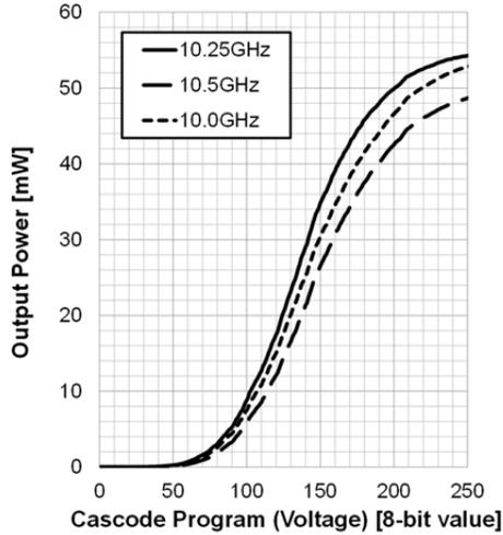
Fig.7: Measured output power over cascode voltage
