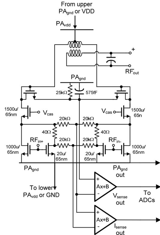
Fig. 3: Circuit detail for PA core, cascode peak voltage and DC current detectors, as well as supply level readout for digitally assisted operation
