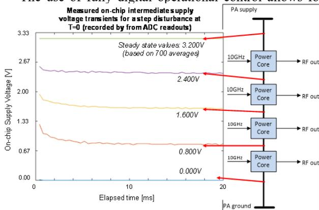
Fig. 5: Measured supply voltage regulation for PSD controller under disturbance at iteration t=0
