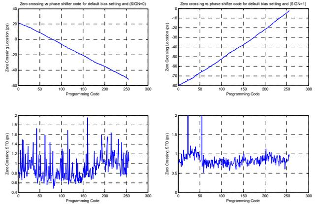
Fig.8: Measured relative signal zero crossing location and standard deviation versus phase program for positive (left) and negative (right) code settings. The absolute crossing times for a programming code of zero coincide for a total of 140ps of timing control.
