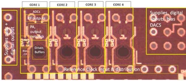
Fig. 4: Die photograph of implemented power amplifier quadrant registers (e.g., for bias voltages). The on-chip RF signal is synthesized and phase-shifted from an input clock at one fourth of the output frequency using on-chip clock multiplier units that consume less than five mA of current while providing digital output phase control.
