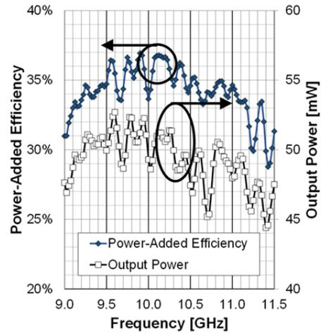
Fig.6: Measured PAE and output power over frequency
