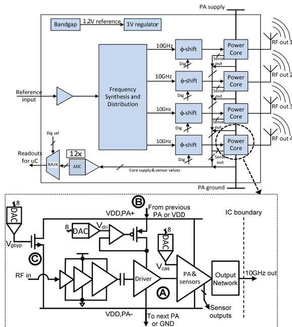
Fig. 1: Simplified block diagram of the integrated X-Band power amplifier quad
