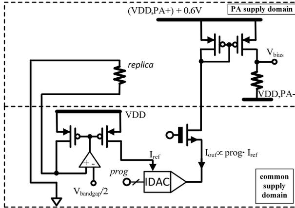
Fig. 2: Bias current generation used for crossing supply domain boundaries. DACs and regulators operate in the common supply domain, providing currents across boundaries to generate voltage offsets proportional to a bandgap voltage in the PA supply domains
