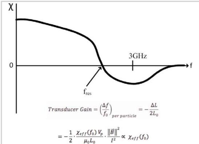
Figure 16.8.1: Typical frequency dependence curve of  $\chi$  for magnetic nanoparticles. Sensor response at each frequency is proportional to  $\chi$  at that frequency.
