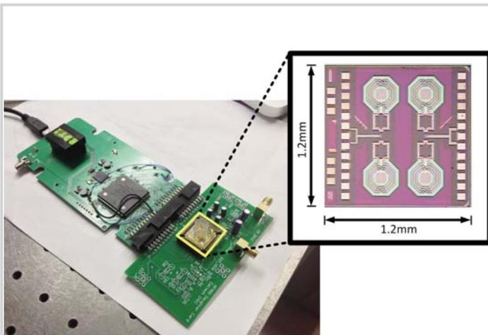
Figure 16.8.7: Handheld USB powered measurement setup with die photo of 2x2 sensor array.
