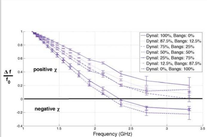
Figure 16.8.5: Spectroscopic measurements of mixtures of various proportions of Dynal and Bangs 1 $\mu$ m beads.
