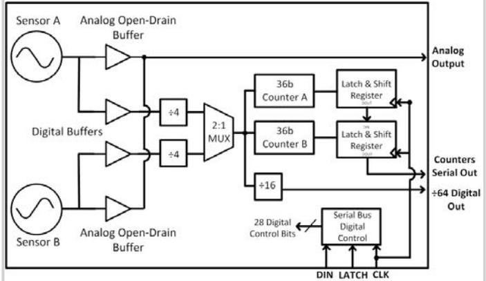
Figure 16.8.2: System block diagram: a 2-sensor unit block is shown, whereas the full implementation has 4 cells.
