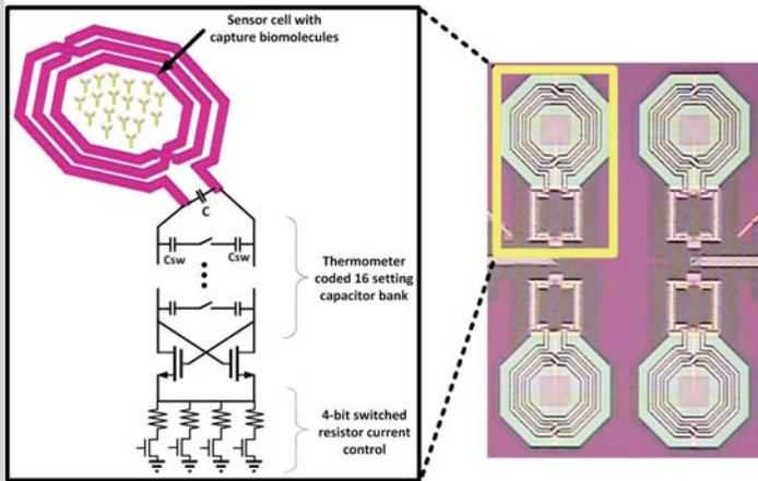
Figure 16.8.3: Sensor cell schematic and die photo.
