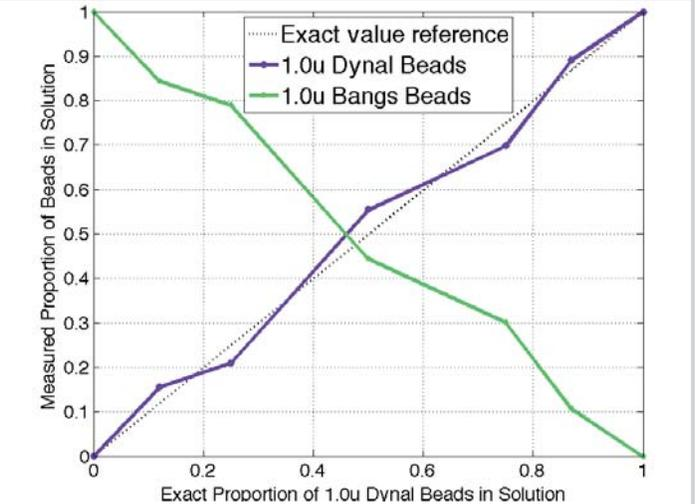
Figure 16.8.6: Measured proportion of beads from data of Fig. 16.8.5 for different ratios: [D%, B%]: 100:0, 87.5:12.5, 75:25, 50:50, 25:75, 12.5:87.5, 0:100.
