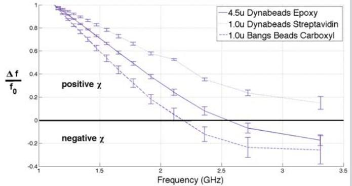
Figure 16.8.4: Frequency response measurement of three different kinds of beads. Error bars represent one standard deviation around the mean across 3 measurements for each bead type.
