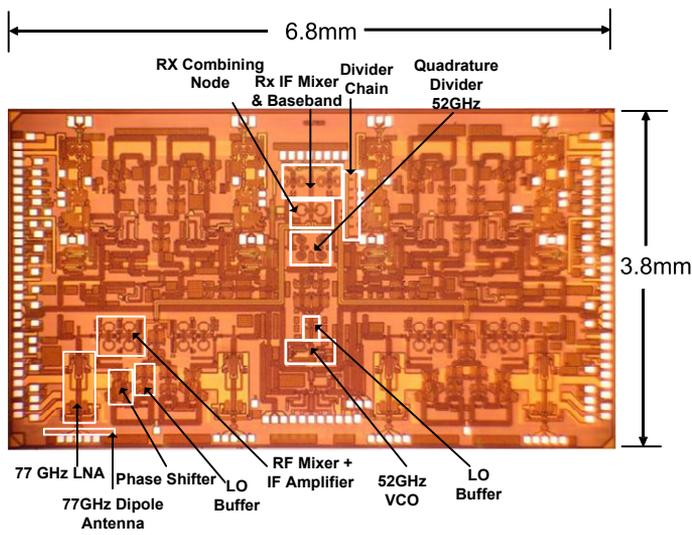
Figure 10.1.7: Chip micrograph.
