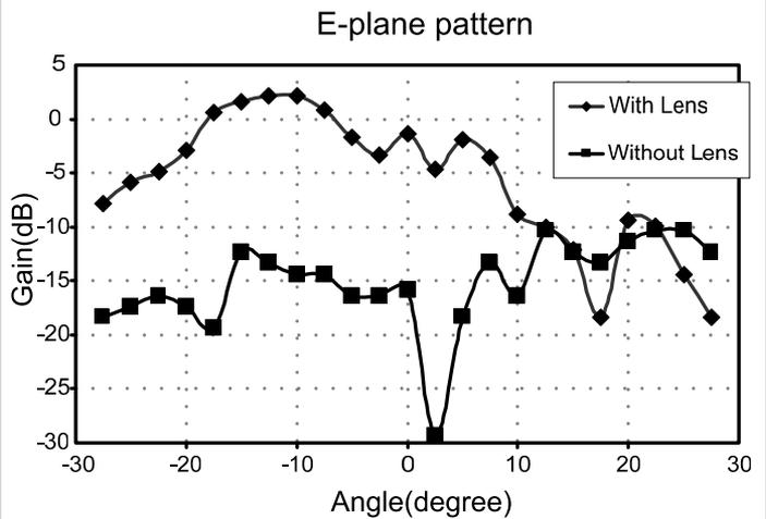
Figure 10.1.6: E-plane pattern of a single on-chip dipole.
