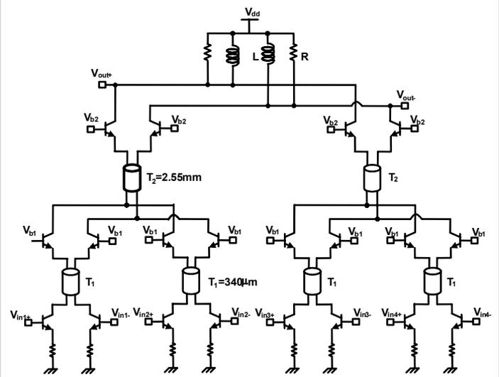
Figure 10.1.4: Schematic of the distributed active phase combining.
