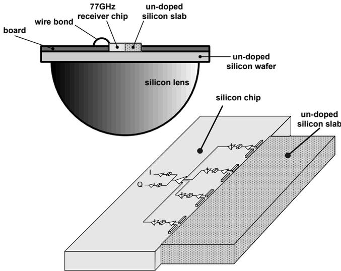
Figure 10.1.1: Chip, board, and lens antenna setup configuration.
