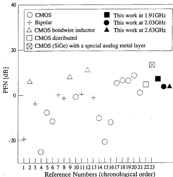
Fig. 23. PFN for various oscillators.
