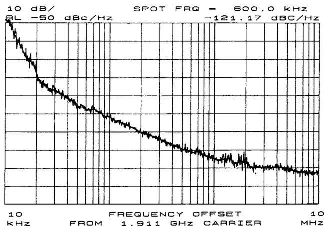
Fig. 22. Measured phase noise versus  $f_{off}$  at 1.91 GHz.
