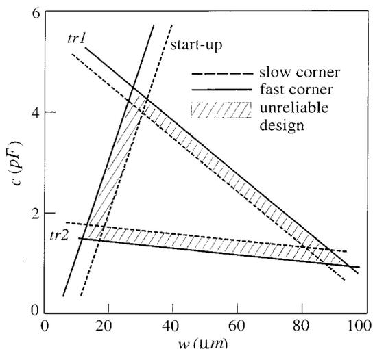
Fig. 15. Process variations and resultant constraint change.
