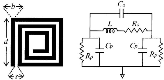
Fig. 7. Symmetric spiral inductor model.
