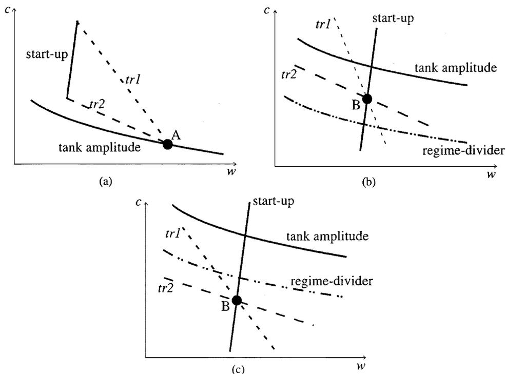
Fig. 14. Design constraints with  $L = L_{opt}$ . (a)  $L$ -reduction limited by the tank amplitude constraint. (b)  $L$ -reduction limited by the startup constraint without waste of power. (c)  $L$ -reduction limited by the startup constraint with waste of power.
