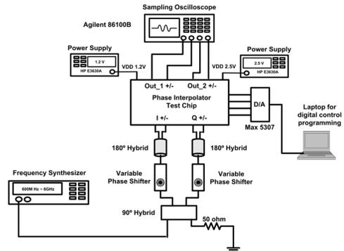
Fig. 10. Measurement Setup for Time Domain Phase Shifting
