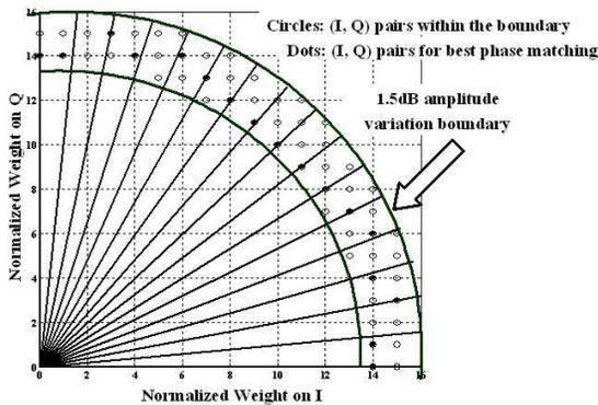
Fig. 3. 10 bit Cartesian Phase Interpolating,  $M=10$  and  $N=6$
