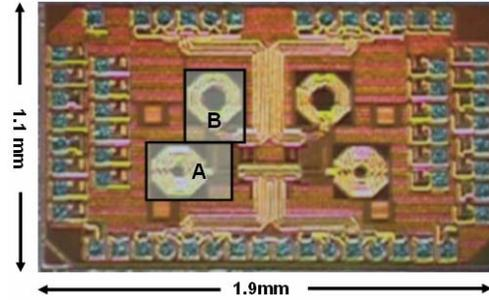
Fig. 9. Die Photograph of the Phase Rotator Chip
