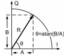
Fig. 1. Vector Diagram of Cartesian Phase Interpolating
