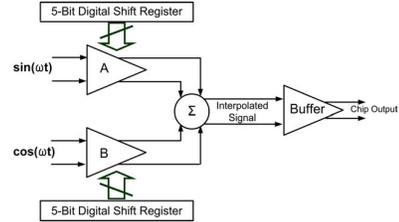
Fig. 5. Block Diagram of Cartesian Phase Rotator
