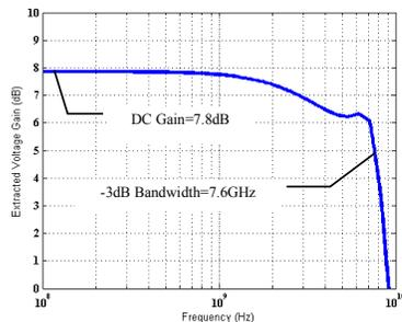
Fig. 13. Extracted Voltage Gain
