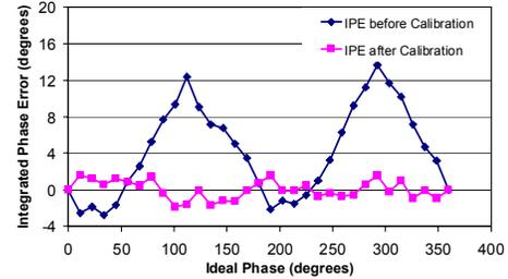
Fig. 14. Calibration for Input I & Q mismatch
