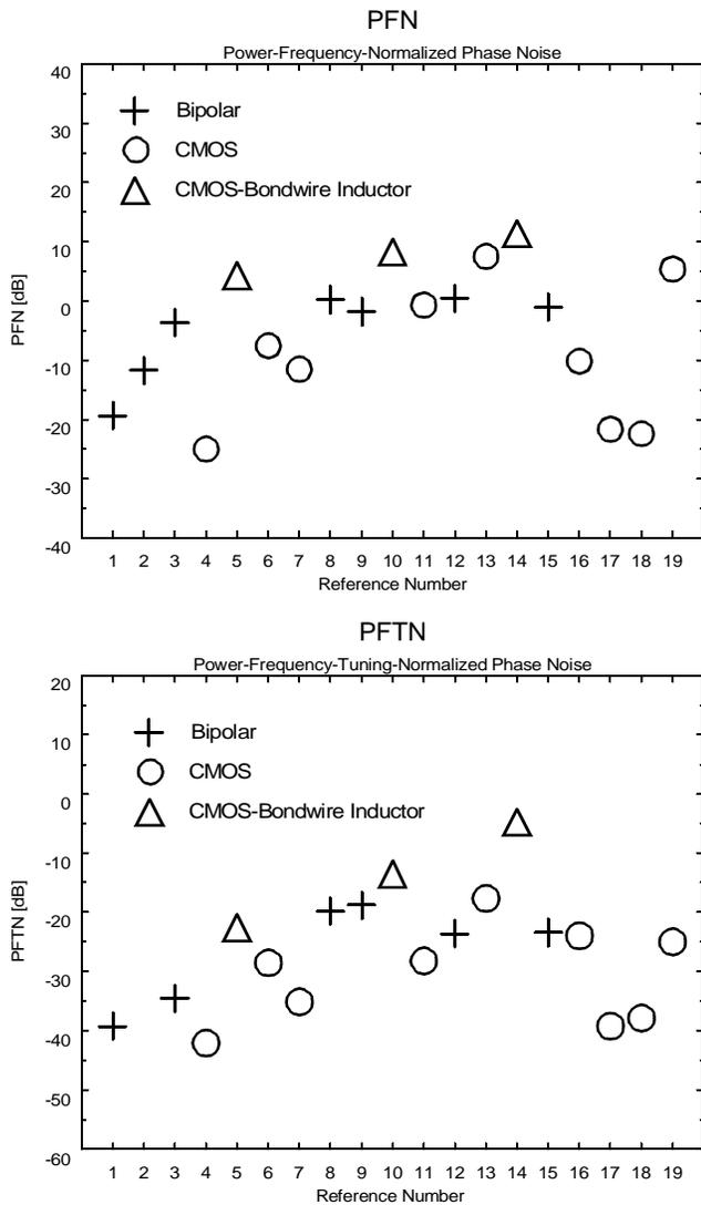
Figure 5  $L_{PFN}$  and  $L_{PFTN}$  for various oscillators.
