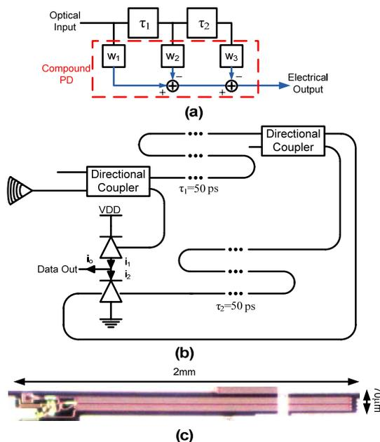
**Figure 1.** Proposed self-equalizing photo detector. (a) Conceptual block diagram, (b) detailed implemented block diagram, and (c) the die photo of fabricated detector
