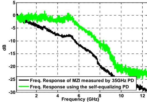
**Figure 2.** Electro-optical frequency response of the channel with a 35GHz PD and with proposed self-equalizing PD. The self-equalizing PD provides up to 7dB of equalization.
