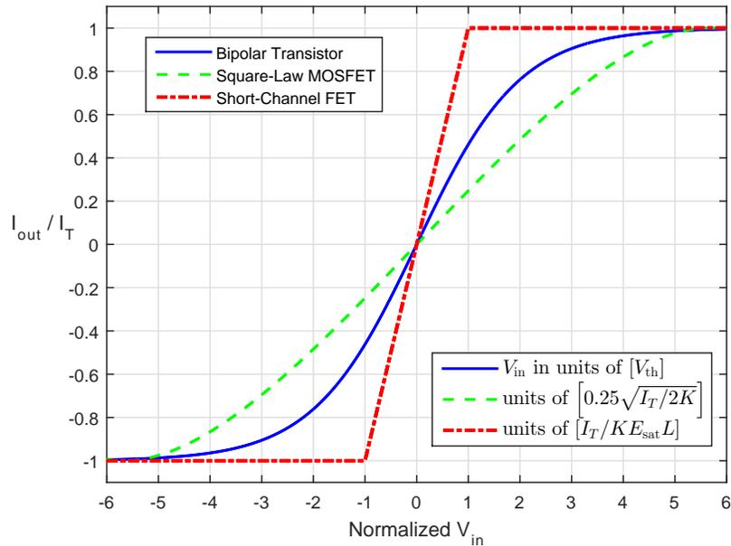
Figure 4: Current switching in a differential pair as a function of the input voltage. Base current and subthreshold conduction were ignored. Due to the chosen normalizations for the  $V_{in}$ -axis, the plot scales may not be *quantitatively* comparable.
