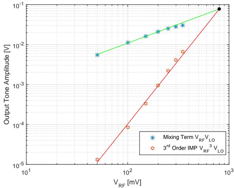
Figure 10: Comparison of fundamental mixing term with third-order IMP. Linear extrapolations on the data were used to obtain the intersection point, which occurs at  $V_{RF}^* = 803$  mV.
