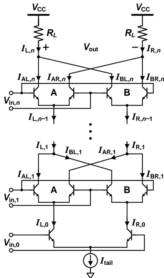
Figure 2: The stacked, balanced, current-commutating analog multiplier. The circuit can also be implemented using field-effect transistors.
