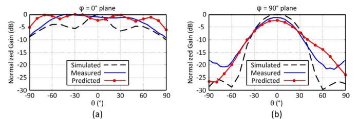
Fig. 7. Normalized simulated, measured, and predicted gain patterns based on PFRS read-outs in (a)  $\varphi = 0^\circ$  and (b)  $\varphi = 90^\circ$  planes for in-phase drive.
