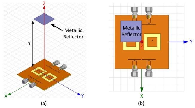
Fig. 4. Simulation setup to investigate the impact of a disturbing metallic reflector on the performance of PFRS: (a) 3-D view and (b) top view.
