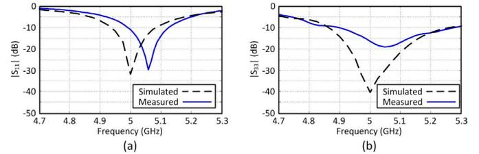
Fig. 6. Measured and simulated input reflection coefficients of (a) the patch and (b) PFRS antennas.
