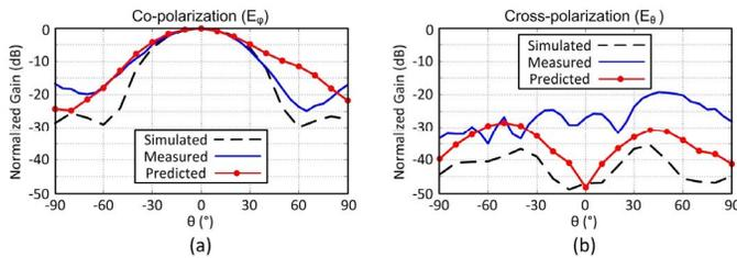
Fig. 9. Normalized simulated, measured, and predicted (a) co-polarization and (b) cross-polarization gain patterns in  $\varphi = 90^\circ$  plane for in-phase drive.
