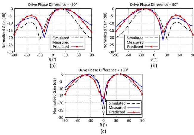
Fig. 8. Normalized simulated, measured, and predicted gain patterns based on PFRS read-outs in  $\varphi = 90^\circ$  plane for (a)  $90^\circ$ , (b)  $-90^\circ$  and (c)  $180^\circ$  of phase difference between the patch antennas.
