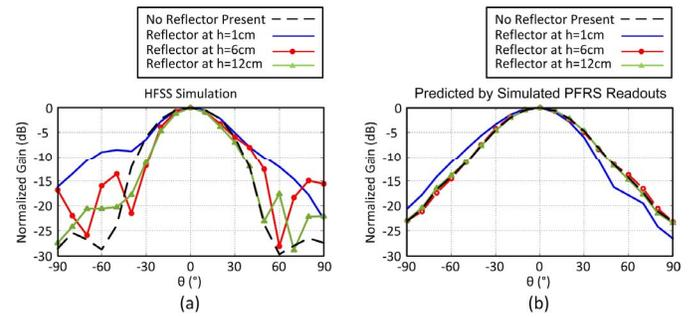
Fig. 5. Comparison of the reflector impact on the normalized gain patterns for  $\varphi = 90^\circ$  plane based on (a) HFSS simulation and (b) prediction by simulated PFRS read-outs.
