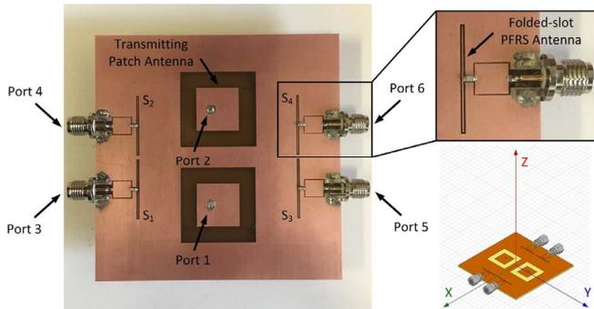
Fig. 2. The prototype PCB antenna array with two transmitting patch antennas and four folded-slot PFRS antennas.
