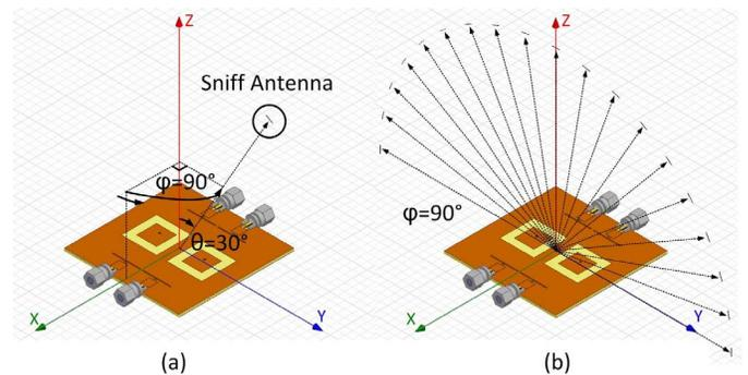
Fig. 3. Simulation setups to relate PFRS read-outs to the polarization of radiated field (a) in an arbitrary direction, and (b) across an entire plane.
