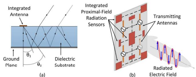
Fig. 1. (a) Generation of surface waves by integrated antenna inside the dielectric substrate and (b) proximal-field radiation sensors that pick up information contained in the excited surface waves.
