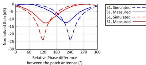
Fig. 10. Measured and simulated amplitude response of  $S_1$  and  $S_2$ .
