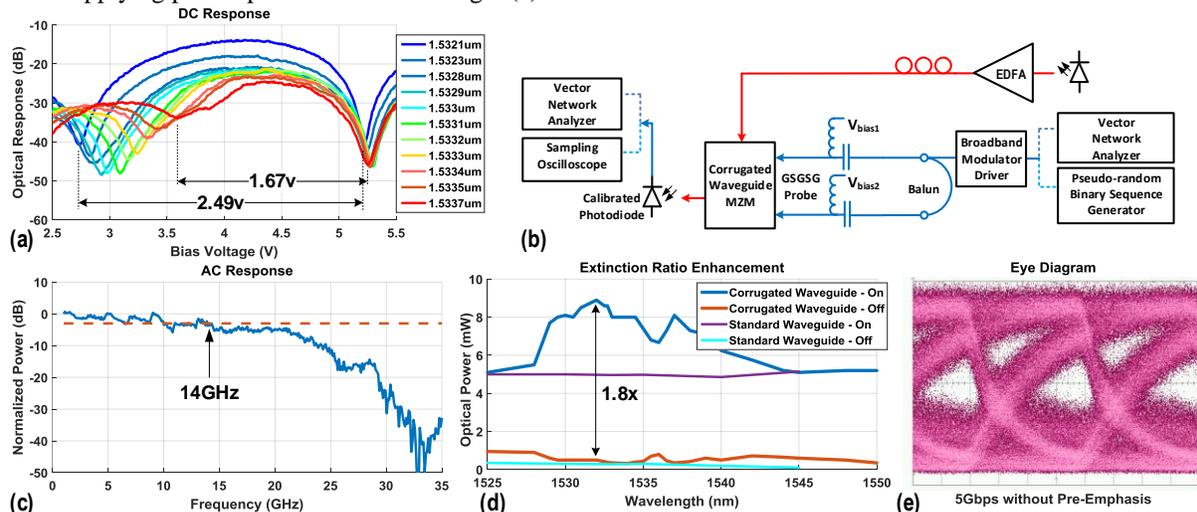
Fig 2. a) DC response of the corrugated waveguide modulator b) Characterization setup c) AC response of the modulator d) Measured extinction ratio of the modulator at 1.25GHz e) Eye diagram for NRZ data transmission at 5Gbps
