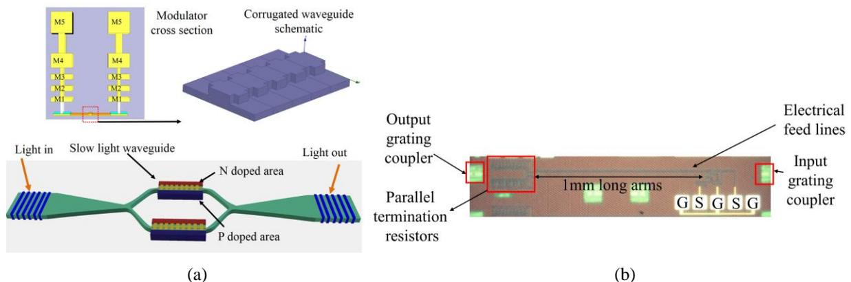
Fig. 1: a) Schematic of the proposed corrugated based slow-light modulator, modulator cross-section view, and schematic of corrugated waveguide b) The die photo of the modulator
