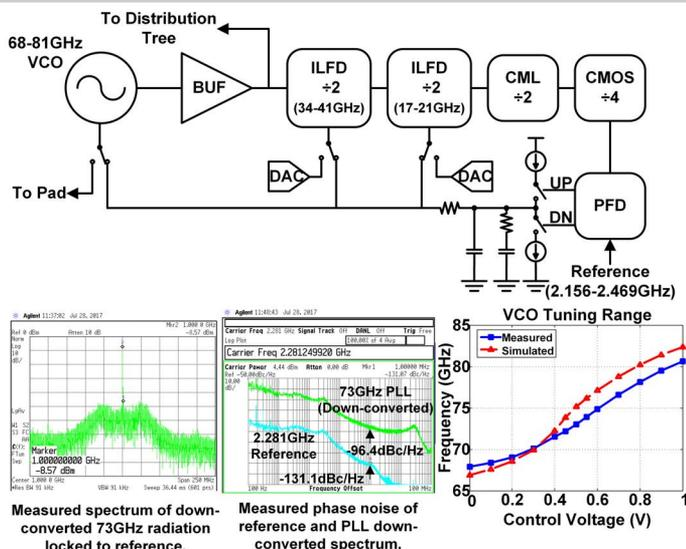
Figure 26.3.3: PLL block diagram and measurement results.
