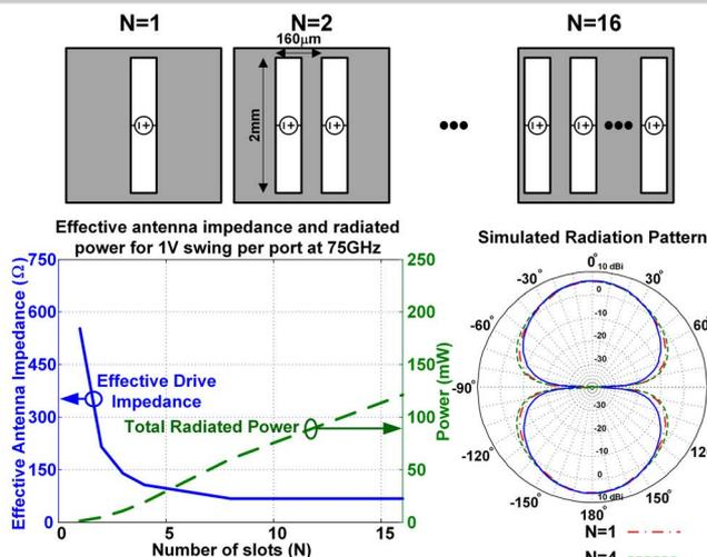
Figure 26.3.1: Impedance- and radiated-power scaling of tightly coupled slot array antennas.
