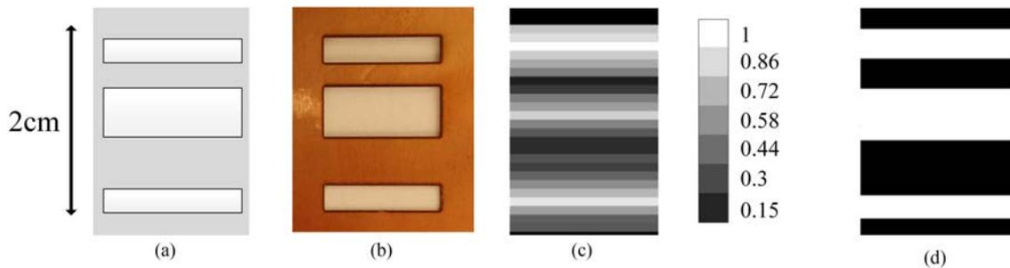
Fig. 11. (a) Barcode design. (b) Fabricated barcode from the copper sheet. (c)–(d) Captured image of the barcode in gray-scale and B&W with the OPA camera.
