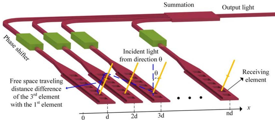
Fig. 1. Conceptual schematic of a 1D direct conversion optical phased array receiver.
