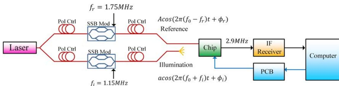
Fig. 7. Block diagram of the measurement setup.
