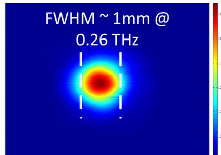
Fig 5. Measured spot size of the focused beam at 0.26 THz on the focal plane.
