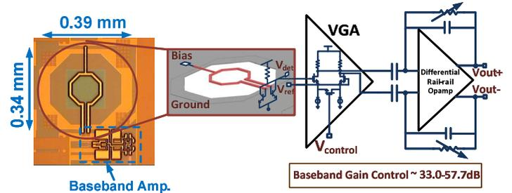
Fig 1. THz imaging receiver in silicon with schematic, integrated antenna, and baseband amplification with 24.7dB tuning range
