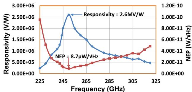
Fig 3. Measured peak responsivity and NEP of the receiver
