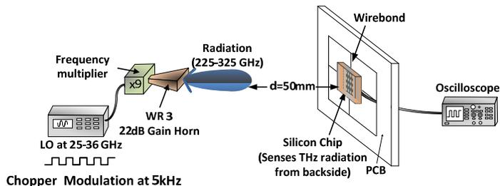
Fig 2. Measurement set-up showing chopped THz radiation captured from the backside of the silicon die
