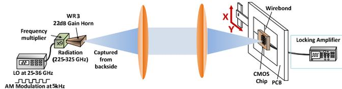
Fig 4. Measurement set-up for focusing emitted THz beam to a diffraction limited spot size on the focal plane which is imaged by the THz receiver by raster-scanning.
