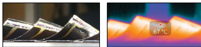
Fig 4. Optical and thermal infrared photographs of the PV concentrator cells operating under simulated AM0 illumination. The cells reach a peak temperature of \sim 70^\circ\text{C} under ambient lab conditions.
