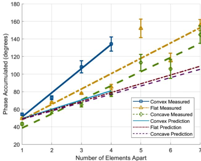
Fig. 6. Shape calibration measurements for bent and unbent array (120 mm bend radius). Linear regression best fit lines are plotted for each of the measured array shapes. Each measured data point represents the average of six separate measurements. The error bars show the standard deviation of the measurement for a given element separation. The convex measurements at element separations above 4 are not included because the bend has moved the elements out of line-of-sight.
