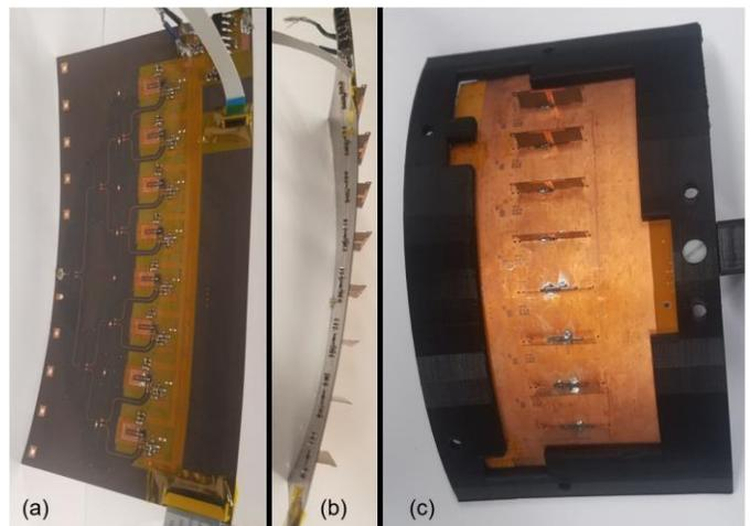
Fig. 1. Flexible Phased Array: (a) Circuit component side of flexible phased array. (b) In-plane view of flexible phased array. (c) Radiator side of flexible phased array.
