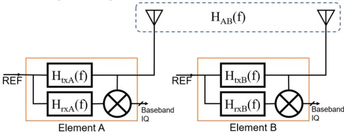
Fig. 4. Simplified calibration model between elements A and B in the same flexible phased array.
