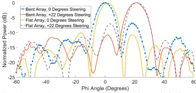
Fig. 5. Beam-steering pattern measurements from  $-60^\circ$  to  $+60^\circ$  for flat and convexly conformed array. Each pattern is normalized to its highest measured value.
