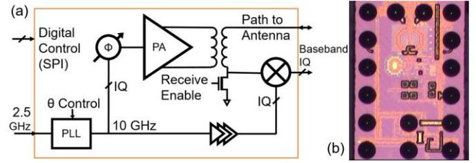
Fig. 3. Transmit/Receive RFIC: (a) Integrated circuit block diagram. (b) Die photo.
